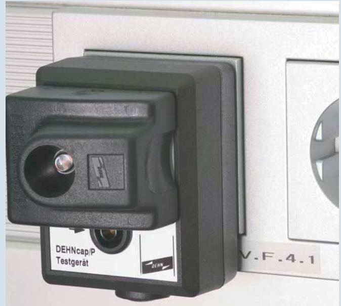
Test unit for testing a DEHNcap/P passive voltage indicator plugged into a 230 V socket outlet for correct operation
