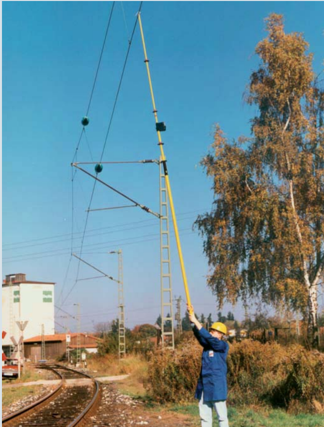
PHE voltage detector with visual indicator used on an overhead contact line of National German National Railways (DB)
