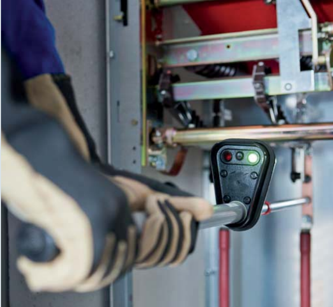
PHE voltage detector with visual indication
