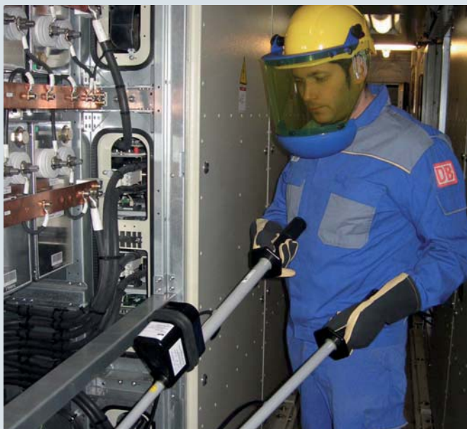
PHE/G II d.c. voltage detector for d.c. links (ICE power car)
