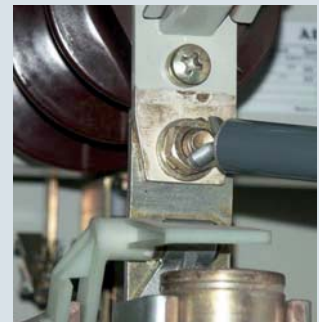
Testing with screwed-on V-shaped electrode
