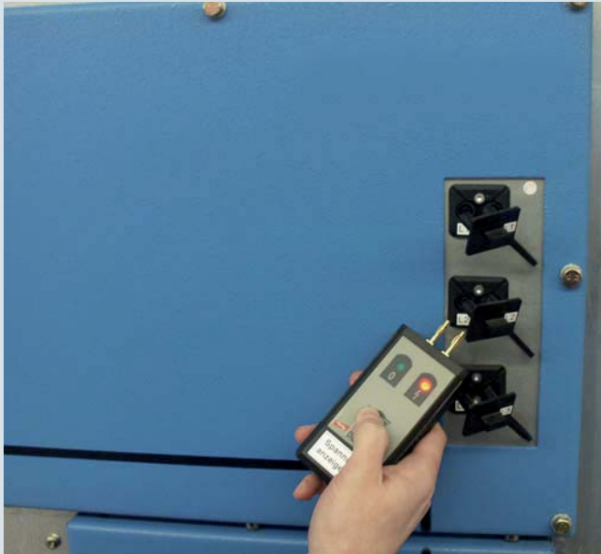
Self-test of a DEHNcap/A voltage indicator
