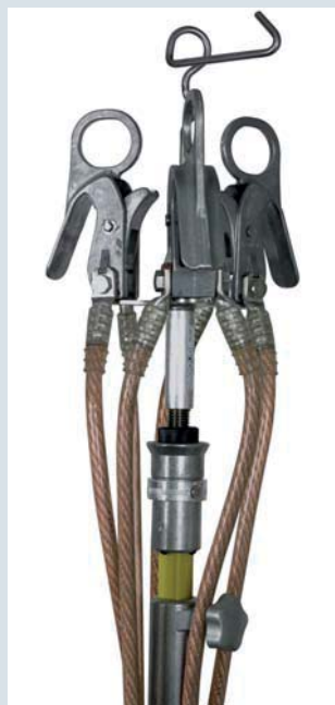
Three-pole coupling aid: with earthing stick (T pin shafts) and lock nut for positioning the coupling aid in the cone coupling.
