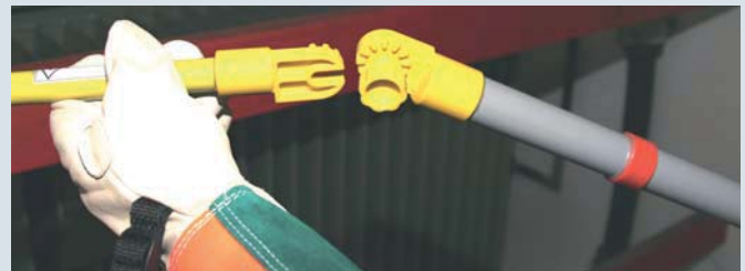
The universal gear coupling permits fast replacement of operating heads and extensions
