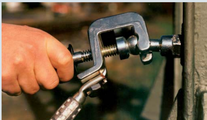
Universal earth clamp with handle connected to a fixed ball point
