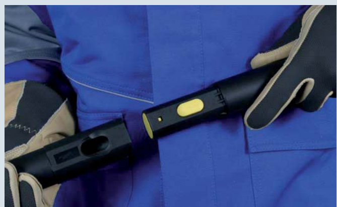
Plugging a HV STK extension handle into an IS PHE STK insulating stick
