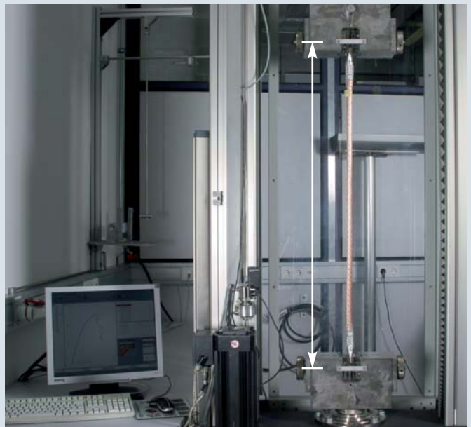
Pull test carried out on an earthing and short-circuiting device
