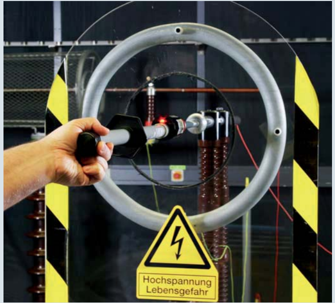
Testing a PHE III voltage detector for immunity to interference fields
