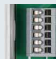
Spring-loaded terminals allow lines to be connected without screws
