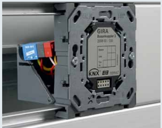
Protection of a KNX bus coupling unit by means of a BUSector surge arrester mounted on a bus terminal in the mounting area of a cable duct.
