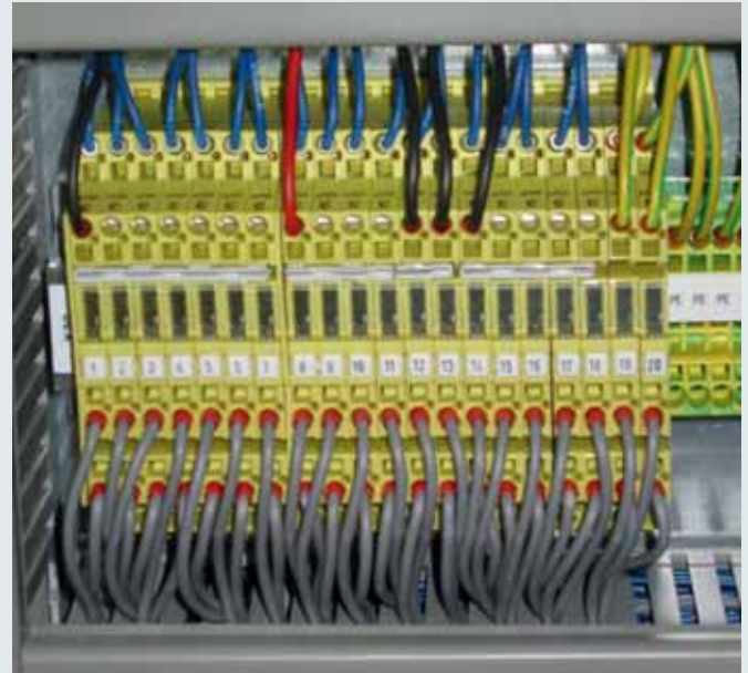
Two-pole terminal block of 6 mm width with integrated surge protection and cage clamp terminal. Earthing via DIN rail or terminal. End plate for the terminal blocks must be ordered separately!
