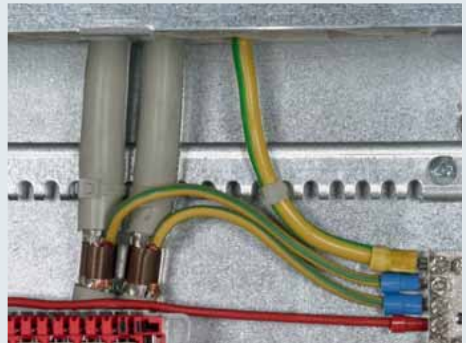
Extremely space-saving shield connection system for use as constant force spring. A spring element compensates the yield of the cable materials.
