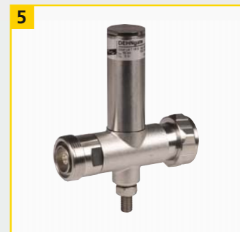
DEHNgate DGA L4 7 16 S Art.-Nr./Part No. 929 047 Kombi-Ableiter in wartungsfreier Lambda/4-Technik mit abgestimmtem Frequenzband. Combined lightning current and surge arrester with maintenance-free quarterwave technology and adapted frequency band.
