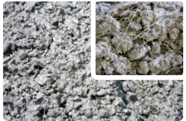
Fresh concrete with steel fibres More information at www.vdsev.de
