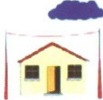
Wire air-termination system
