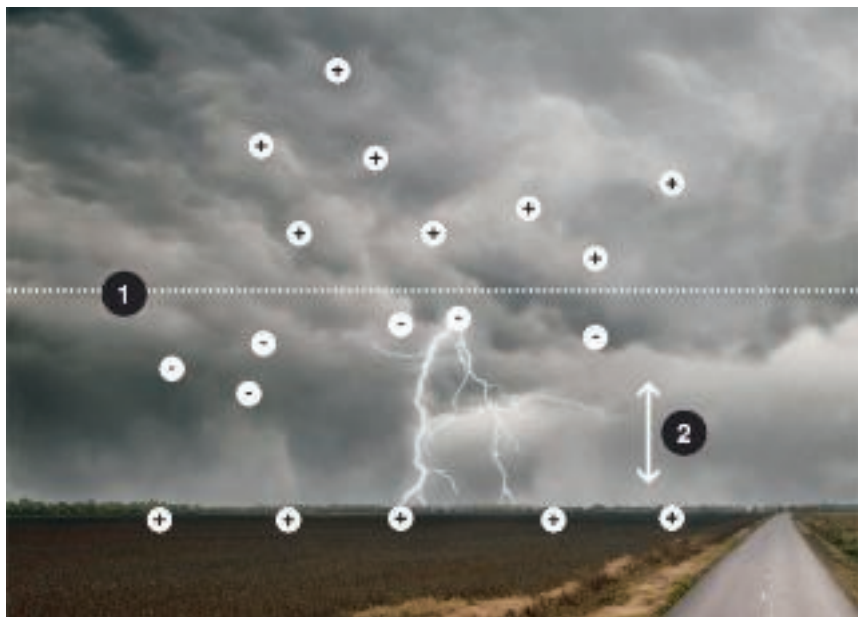
Charge distribution: 1 = approx. 6,000 m, 2 = Electrical field
