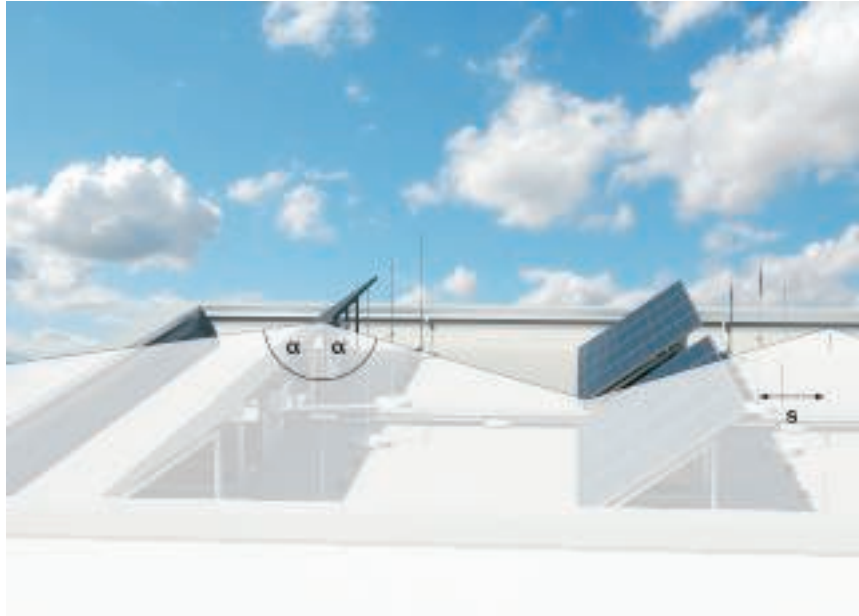
\alpha^\circ = lightning protection angle, s = separating distance
